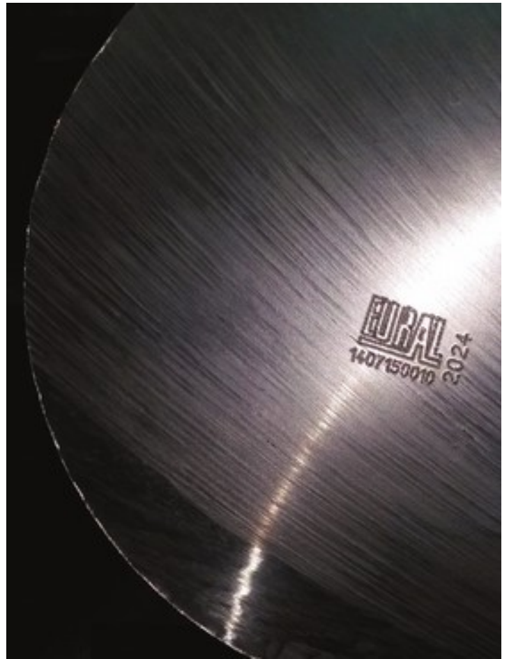
Imprint of Eural logo, alloy code and batch number on all extruded bars
